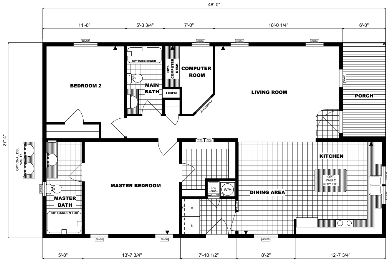
FLOOR PLAN G-3154 28X48 w/6'-0" PORCH TWO BEDROOM, TWO BATH APPROX. 1238 SQ. FT.
